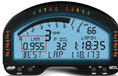
Powering **MXL QM** and Lambda controller on at the same time, **LCU-ONE CAN** is recognised at start-up and probe warm-up procedure starts. During this period the controller takes the probe to its working temperature (until around 780 °C – 1436 °F).
