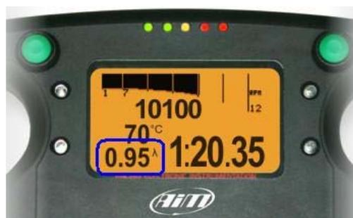
Switching **EVO3 QM** on Lambda controller is recognised at start up and probe warm-up procedure starts. During this period the controller takes the probe to its working temperature (until around 780 °C – 1436 °F).
