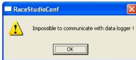
Please, ensure that the data logger is switched on and correctly connected to the PC and then retry to transmit the configuration.
