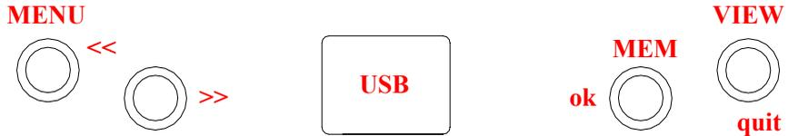
The Keyboard is composed of four push-buttons and it is used to configure the instrument, to recall recorded data and to clear the internal memory.
