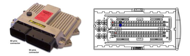
Here below is connection table. As said before the ECU has two CAN lines: CAN0 and CAN1; AiM suggests to use CAN1.
