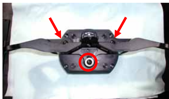
Figure 6: screws that fixes the stock dash
