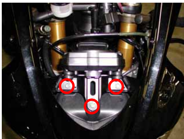
Figure 5: the screws that fix the stock dash to an internal chassis
