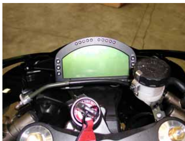
Figure 10: MXL correctly installed.
