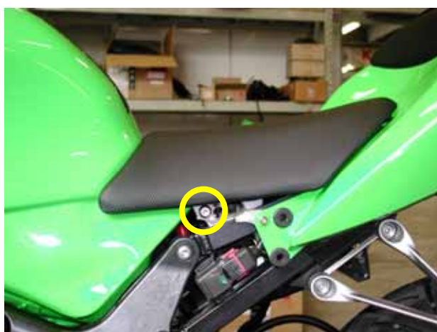
Figure 13: the screw that fixes the seat to the bike.
