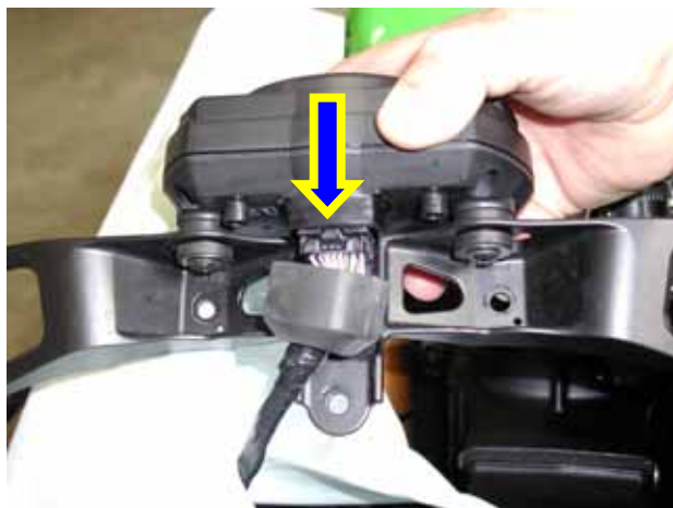
Figure 5: the on board wiring connector
