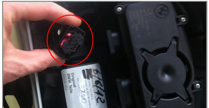
Connect AiM wiring to BMW wiring as highlighted on the right.
