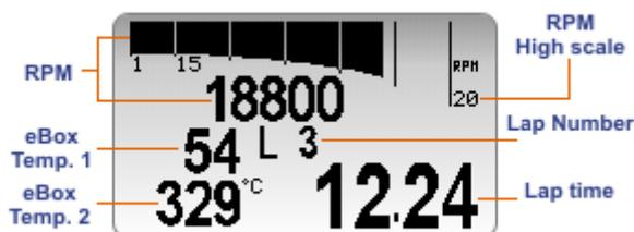
Pressing “ON/VIEW” the display shows speed in spite of RPM digital value (below).
