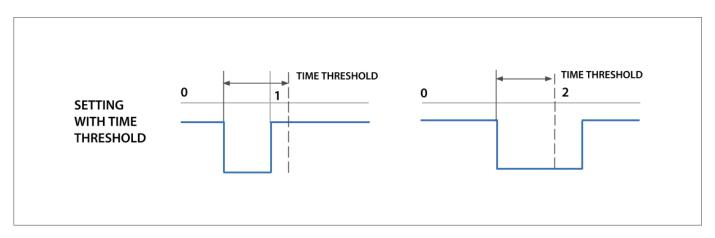
To do so, enable the "use timing" checkbox on the top box of the setting panels. In this case, the pushbutton is set at two different values that you may define according to how long you push it.
