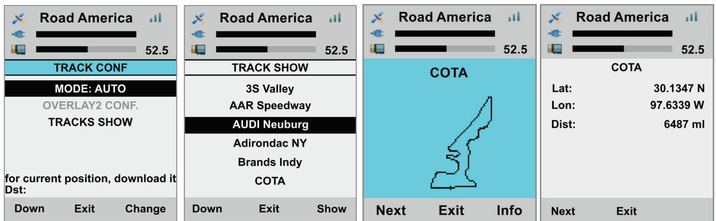
To switch to **MANUAL** mode press “Change” in Auto mode (left image here above) and “MODE: MANUAL” enables.
