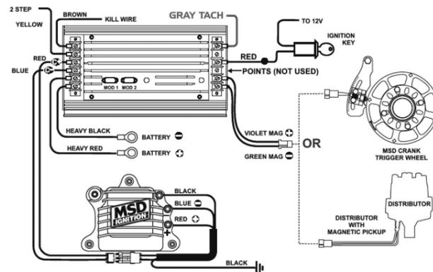
The output labelled "GRAY TACH" gives a 5-50V output that can be directly sampled by Solo 2 DL. In case the vehicle ignition system has no output you need to connect Solo 2 DL to the low voltage of the coil as shown in the following images.
