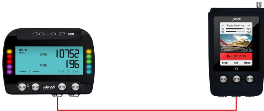
To connect Solo 2 DL to LCU-One CAN connect 5 pins Binder connector placed bottom left of Solo 2 DL to 5 pins Binder connector of LCU-One as shown here below.
