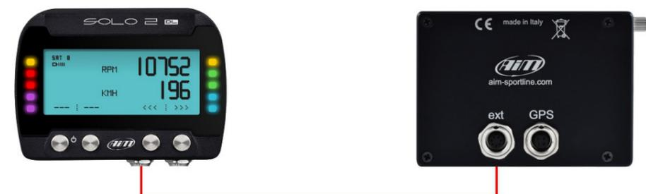
To connect Solo 2 DL to SmartyCam GP HD use SmartyCam CAN cable and connect 5 pins Binder connector placed bottom left of Solo 2 DL to 7 pins central Binder connector of SmartyCam HD as shown here below.
